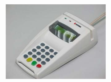
ESL850 is a multifunction card reader & writer which perfectly combine the function of magnetic card reading, IC card / SAM card reading & writing and also customer personal information & password inputting, build standard hardware platform for reading/writing contact logic encryption card and COS operation of CPU card.
